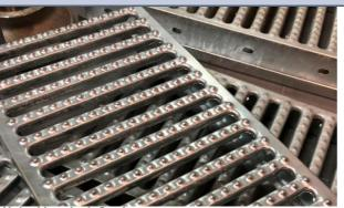
United Interlock Grating Those items fills a multitude of needs including florring and walkways.mezzanines,stair treads,maintenance and staging platforms,scaffolding planks,archetectural wall coverings and more. Material: Carbon Steel Finish: HDG Anti-skid,slotted-smooth punched surface and solid unpunched surface. Double male and male-female leg shapes.
